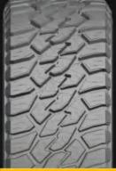
\*The outside blocks are designed for extended wear with an aggressive look. \*Designed with an optimized void ratio to allow for a high surface area, improving mud traction and promoting long, even tread wear, while effectively cleaning out rocks in off-road conditions.
