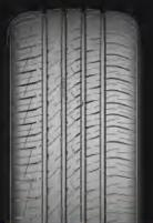
\*Four main groove design provides excellent drainage performance;
